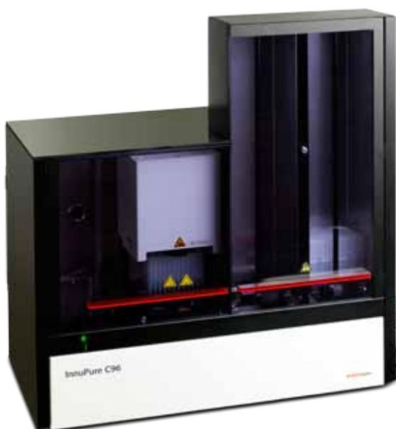
▲ The InnuPure® C96 a compact and fully automated nucleic acid extraction system for up to 96 samples
